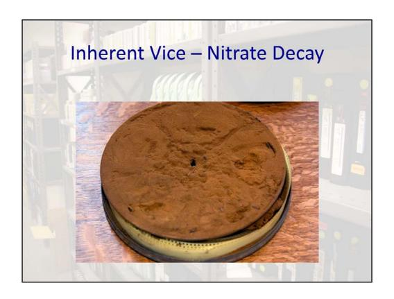
•This is a nitrate film in a late stage of nitrate breakdown. This illustrates how some kinds of AV media were not necessarily built to last.
