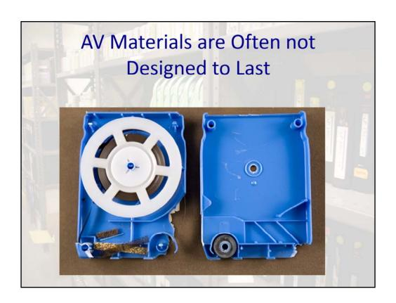
•This detail of the guts of an 8-track tape shows the deterioration of the sponge (lower left) that supports the tape itself as the cartridge is being played back. This sponge dries out over time and falls apart, leading to faulty playback and contamination of the tape itself with the sponge material.
